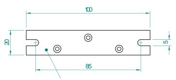
Mounting Flange to Heatsink Apply Thermal Compound Max. Temp 70deg C
